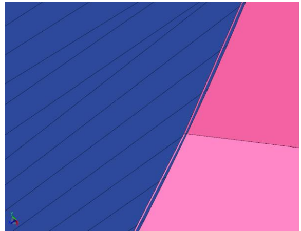
Figure 4. Dirty CAD with a small gap not fully sealed
